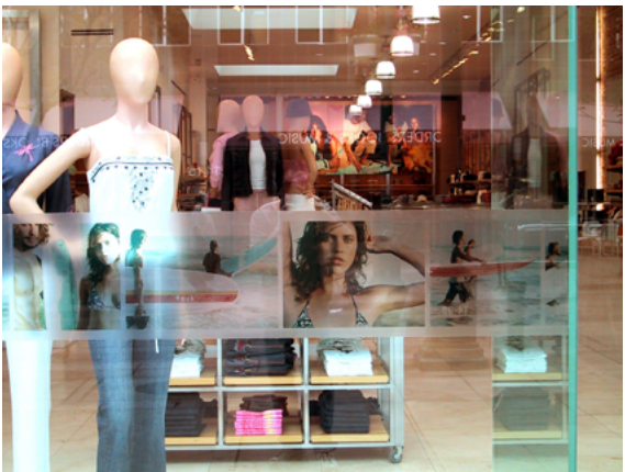
Window Graphics: Translucent film with muted coloration is applied directly to storefront glazing.
