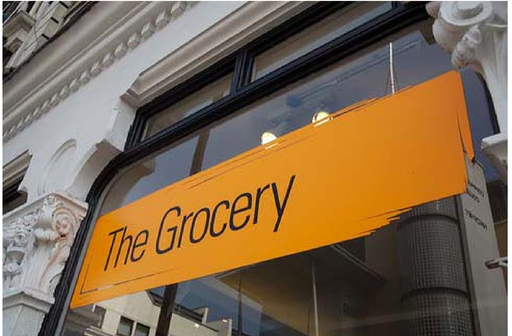
Window Graphics: Color printed directly on glass with letterforms dropped out to create transparency.
