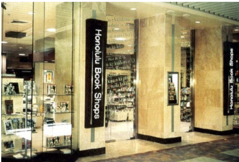
Primary Sign: Metal face box with internal illumination and push-through acrylic letterforms. Cabinet style construction will be considered on a case-by-case basis.
