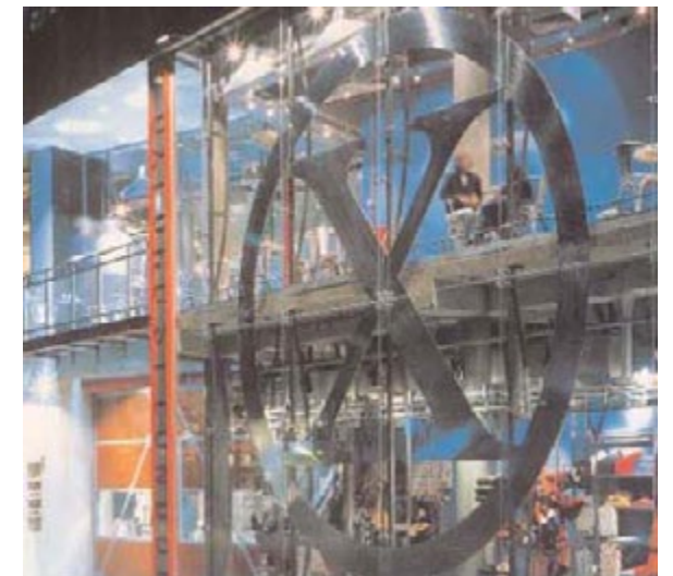
Secondary Sign: Laser cut metal with polished, finished edges.
