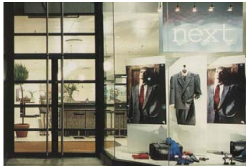
Primary Sign: Metal face with internal illumination and push-through acrylic.
