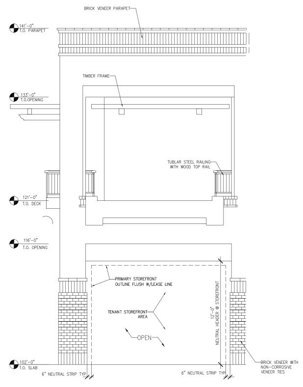
VARIES TO, PARAPET WALL MOUNTED BLADE SIGN TO DECK 0'-0'
