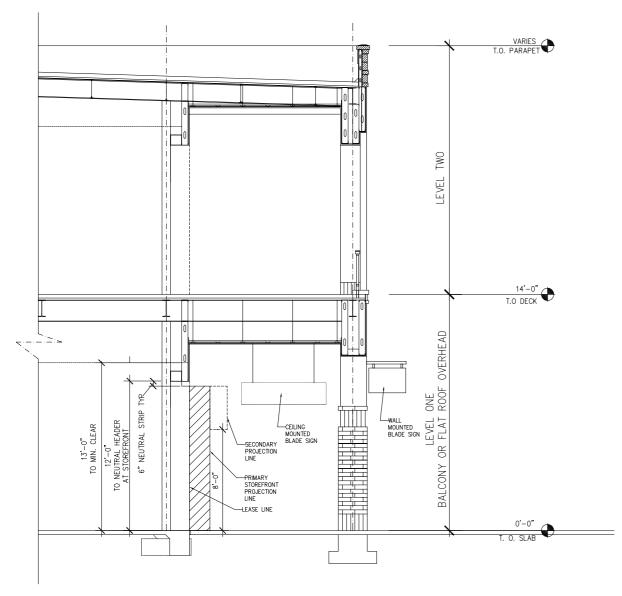
COLUMN CENTER LINE STRUCTURAL COLUMN BY LANDLORD NEUTRAL PIER BY -LEASE LINE -PRIMARY STOREFRONT PROJECTION LINE -SECONDARY PROJECTION LINE ABOVE 6" NEUTRAL STRIP TYP 1'-0" 30'-0" STRUCTURAL PIER® BALCONY OR FLAT ROOF OVERHANG BY LANDLORD —LINE OF BALCONY OR FLAT ROOF OVERHANG ABOVE BY LANDLORD
