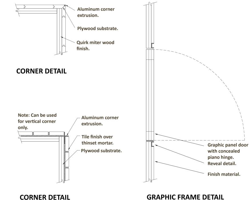
Note: For interchangable frameless graphic panels, change graphic from back via concealed hinges and reveal details. (for back lit panels as well to replace lights). Use concealed / magnet activated locks to secure door.
