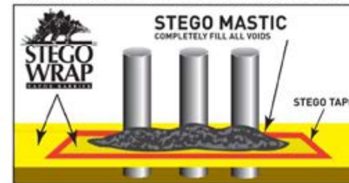
FIGURE 5: MULTIPLE PIPE PENETRATION SEALING
