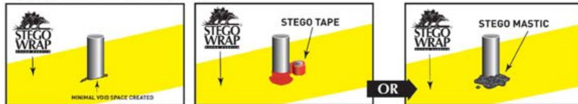
FIGURE 4a: PIPE PENETRATION SEALING
