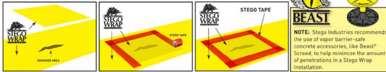
FIGURE 3: SEALING DAMAGED AREAS
