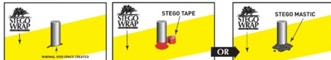
FIGURE 4a: PIPE PENETRATION SEALING
