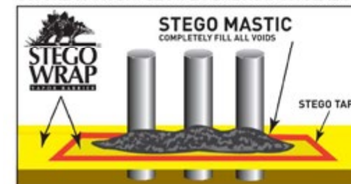
FIGURE 5: MULTIPLE PIPE PENETRATION SEALING
