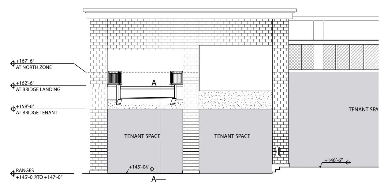
A - WEST ELEVATION OF BUILDING 3 AT PEDESTRIAN BRIDGE
