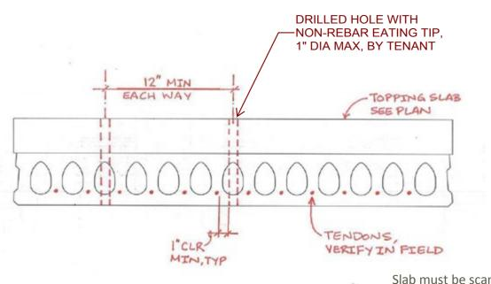
NOTE: DO NOT DAMAGE TOPPING SLAB REINFORCING. CONTRACTOR TO LOCATE REINFORCING & TENDONS PRICE TO DRILLING Slab must be scanned prior to any core drilling to ensure compliance with coring guidelines.
