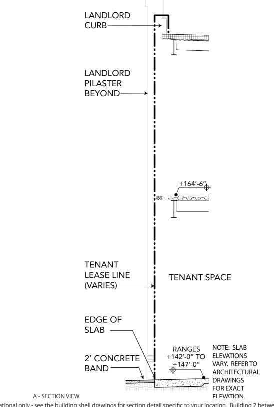
This section is representational only - see the building shell drawings for section detail specific to your location. Building 2 between grid lines 3-5 does vary from these details shown
