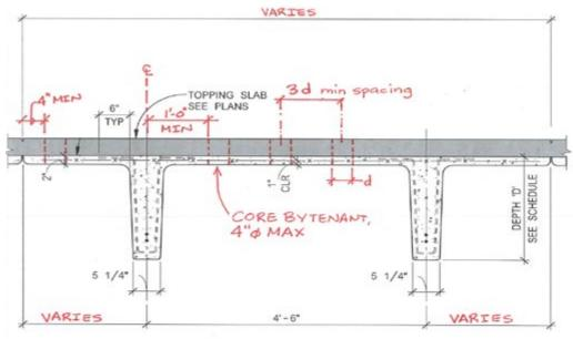
NOTE: DO NOT DAMAGE TOPPING SLAB REINFORCING. CONTRACTOR TO LOCATE REINFORCING PRIOR TO CORE DRILLING. NOT TO EXCEED 4 CORES IN ANY 4'-0"X4'-0"AREA. Slab must be scanned prior to any core drilling to ensure compliance with coring guidelines.
