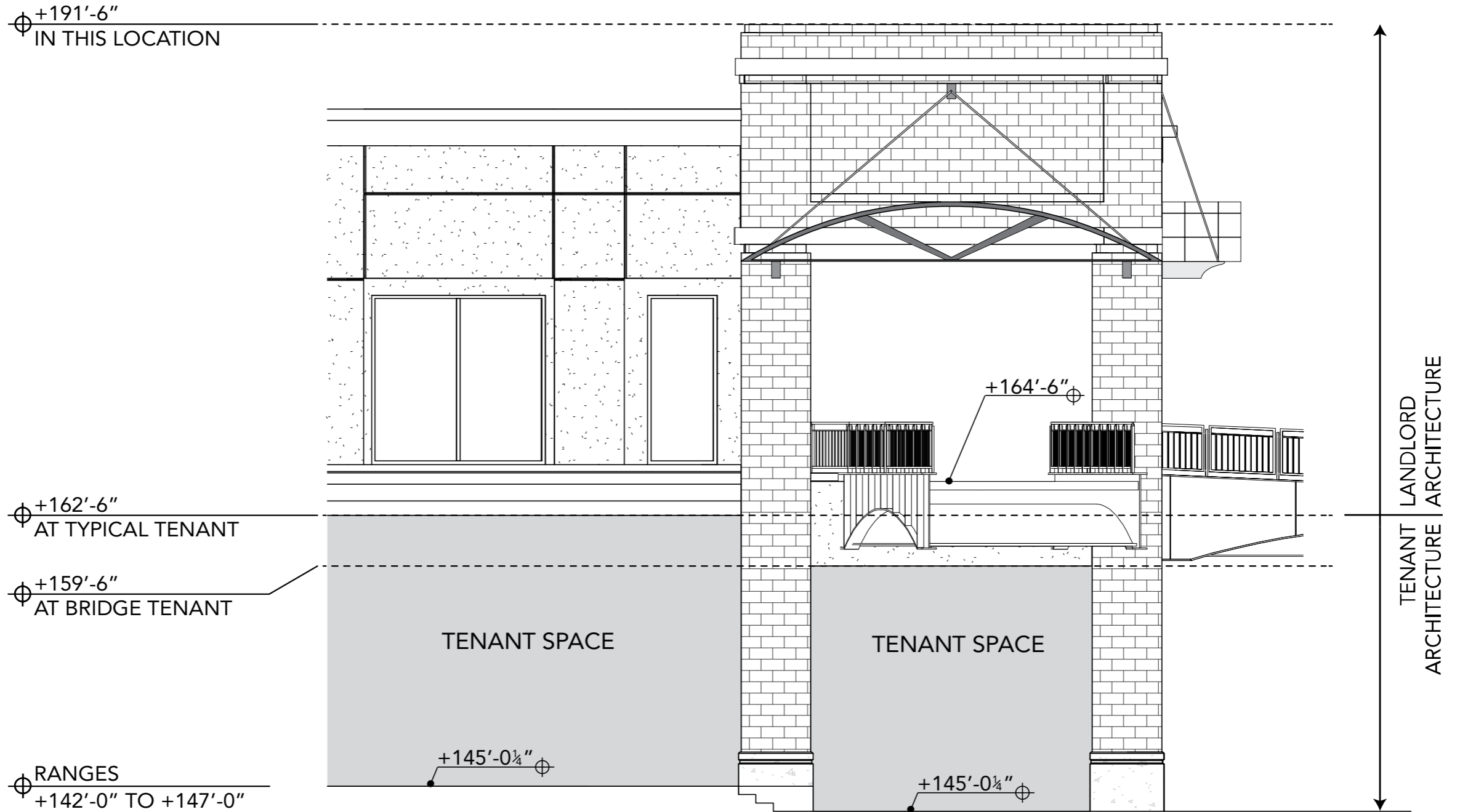
A - EAST ELEVATION OF BUILDING 2 AT PEDESTRIAN BRIDGE
