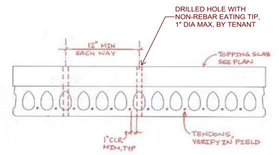
NOTE: DO NOT DAMAGE TOPPING SLAB
