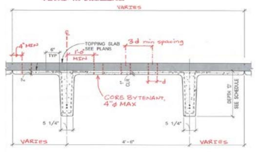
NOTE: DO NOT DAMAGE TOPPING SLAB
