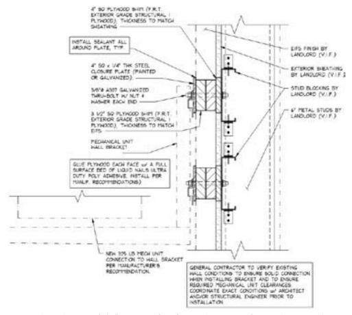
Minimum head clearance of 6'-8" is required from floor to lowest point of RTU bracket assembly.
