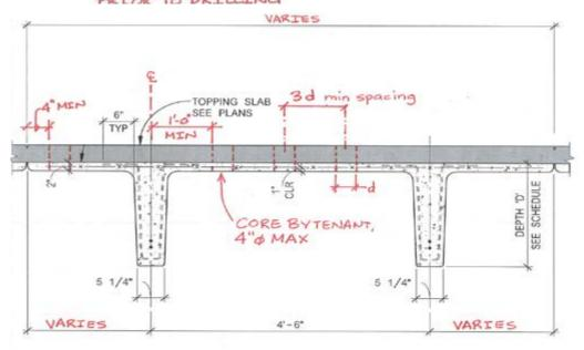
NOTE: DO NOT DAMAGE TOPPING SLAB
