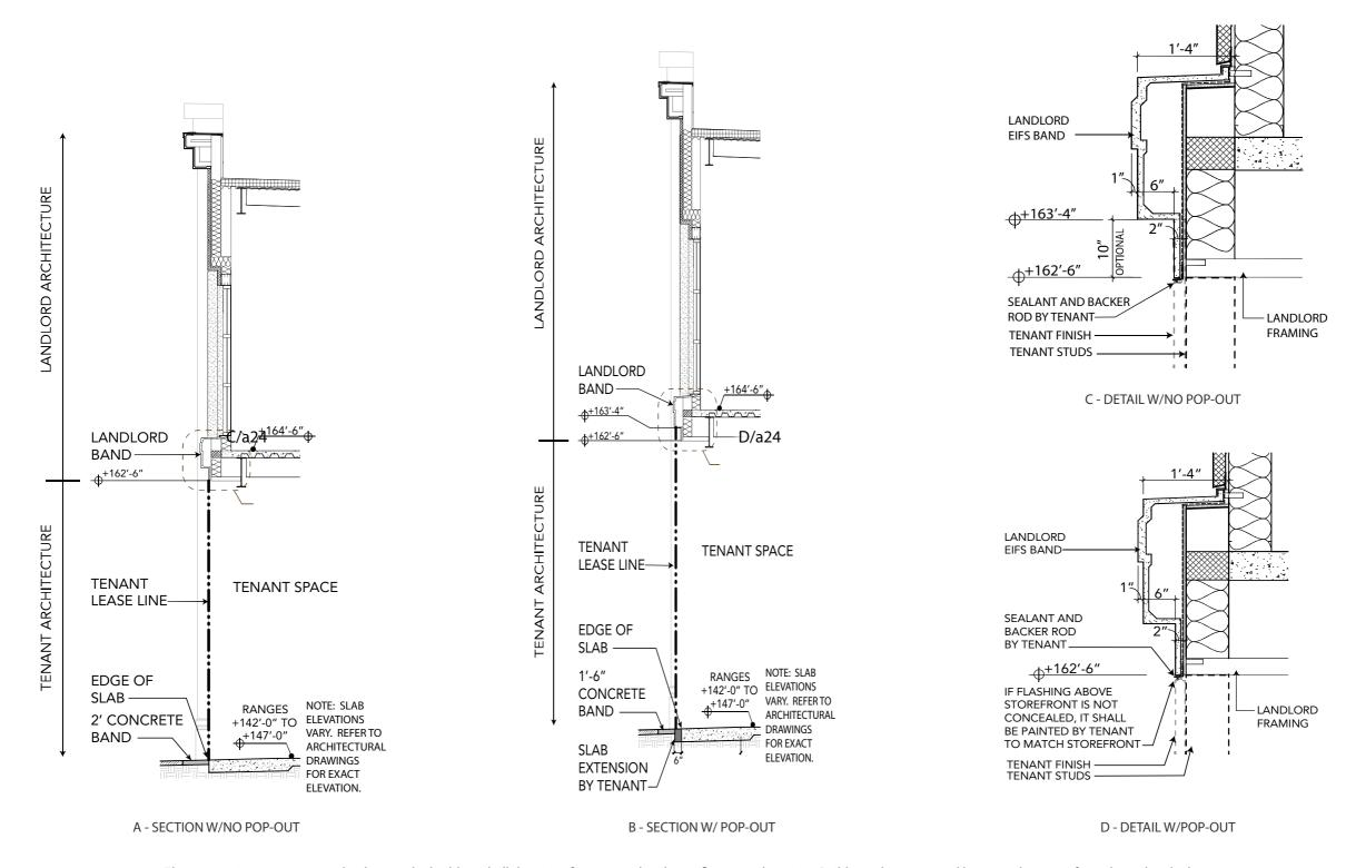
This section is representational only - see the building shell drawings for section detail specific to your location. Building 2 between grid lines 3-5 does vary from these details shown
