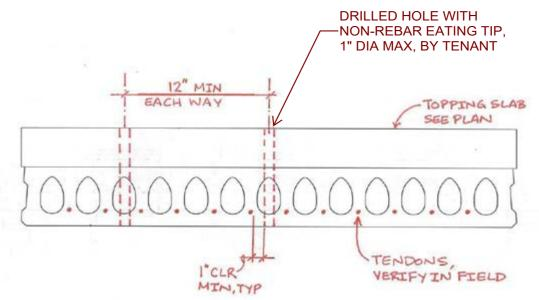
NOTE: DO NOT DAMAGE TOPPING SLAB
