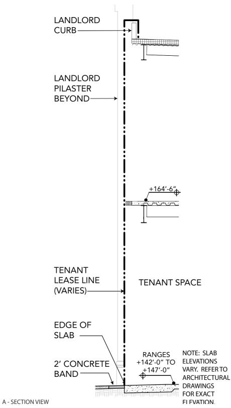
This section is representational only - see the building shell drawings for section detail specific to your location. Building 2 between grid lines 3-5 does vary from these details shown
