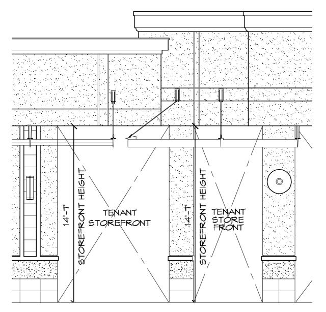
ALL DIMENSIONS TO BE VERIFIED IN FIELD. Required storefront height at 14'-7". If LL trellis is existing, Tenant is allowed to have sign mounted on trellis.
