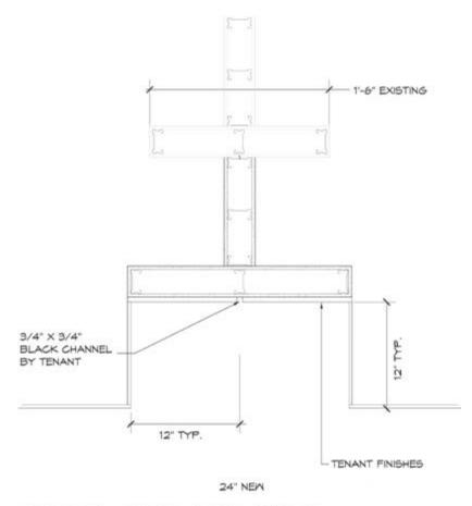
PLAN DETAIL @ NEUTRAL CHANNEL CONDITION SCALE: NTS
