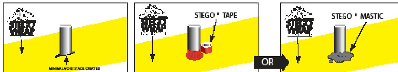
STEGO WRAP PIPE PENETRATION REPAIR DETAIL:
